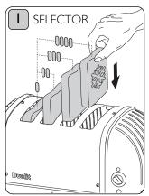
Rotate the 'selector switch' clockwise to the desired number slots you require and insert your frozen slices of bread.
